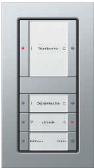
Gira Tastsensor 2, 4fach, transparent Gira push button sensor 2, 4-gang, transparent
